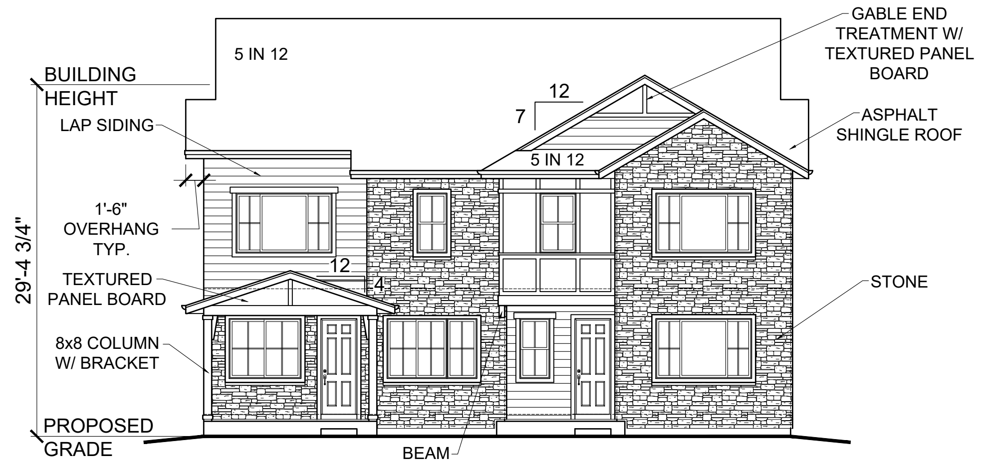
PLAN 1 & 3 ELEVATION 'B' - FRONT 58% MASONRY PROVIDED AT FRONT SCALE: 1/8" = 1'-0" 30% MASONRY AVERAGE TOTAL (30% REQ.)
